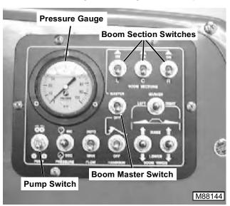
5. Move pump switch to ENGAGED position. This will engage the pump clutch.
