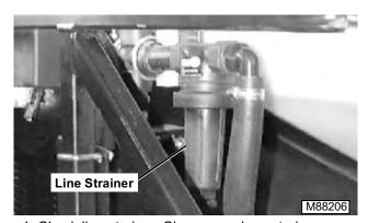
Check line strainer. Clean or replace strainer element as needed.
